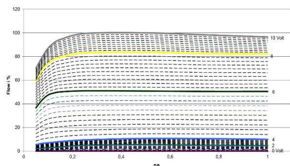
Pressure Independence Curves: FlowCon PICV with Modulating 0-10V Actuator
