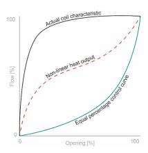
Actual McQuay MCM-DW Coil Characteristic: Non-linear Heat Output with Equal% Control
