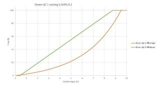
Control Curves: FlowCon Green.0 or Green.1 with FN-actuator (Linear and Equal% Control Mode)
