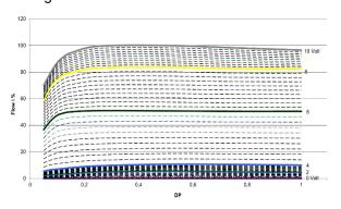
Pressure Independency Curves: FlowCon PICV with Modulating 0-10V Actuator
