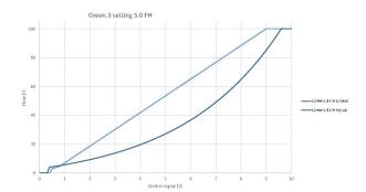
Control Curves: FlowCon Green.3 with FH-actuator (Linear and Equal% Control Mode)
