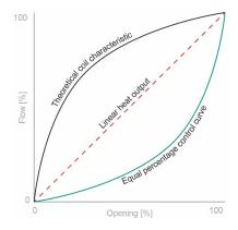
Theoretical Coil Characteristic: Linear Heat Output with Equal% Control
