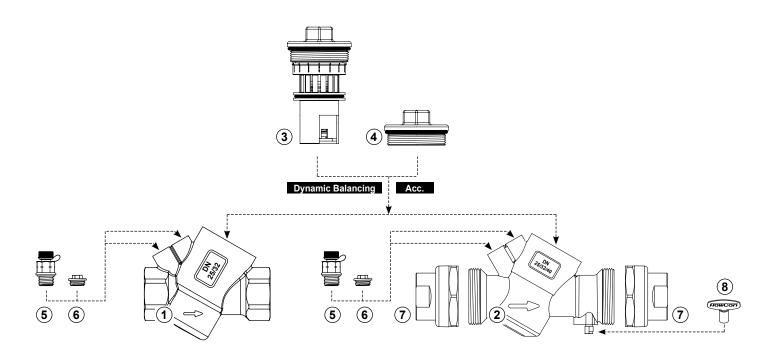
FlowCon Composite Insert DN25-40 (1"-1 1/2") · Dynamic Balancing Valve
