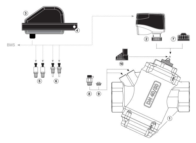
FlowCon FIT-G.3 DN40-50 (1 1/2"-2") · Pressure Independent Temperature Control Valve
