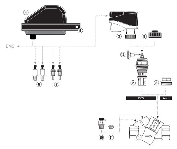
FlowCon FIT-G.0/1 DN15-25 (1/2"-1") · Pressure Independent Temperature Control Valve
