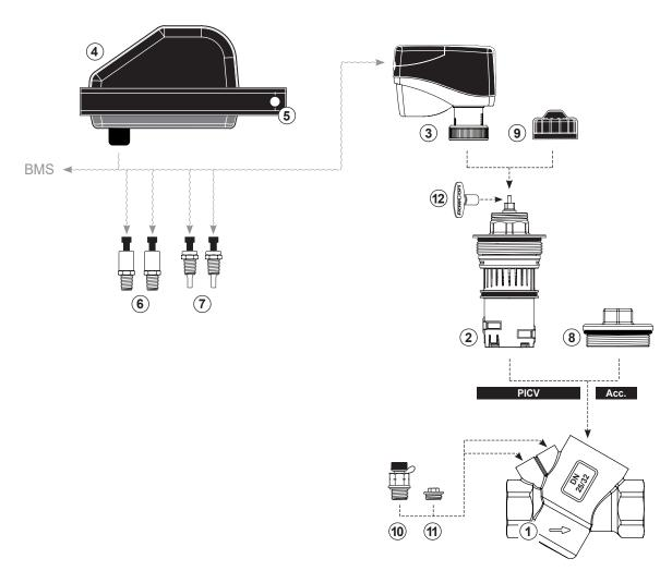
FlowCon FIT-G.2 DN25-32 (1"-1 1/4") · Pressure Independent Temperature Control Valve
