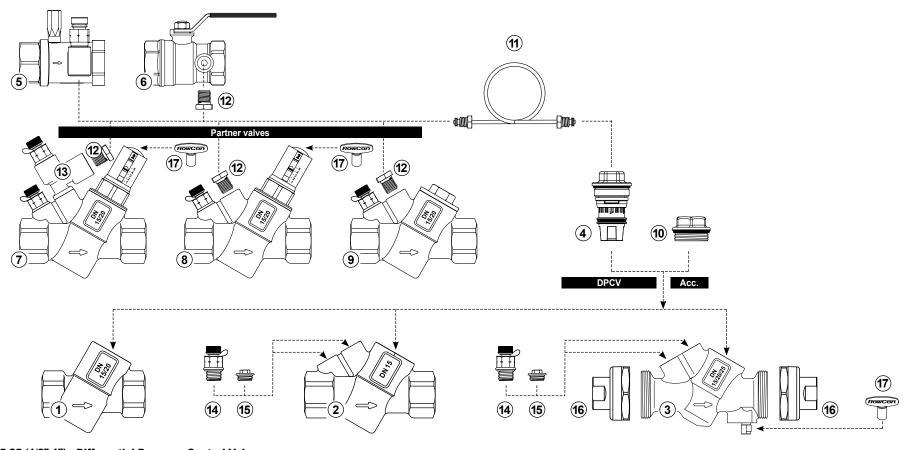
FlowCon SDP DN15-25 (1/2"-1") · Differential Pressure Control Valve
